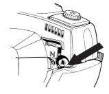
Choke: Set the choke control in the choke position.
